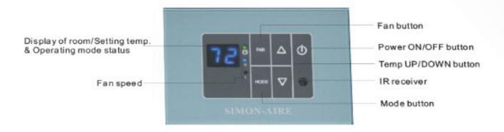
Power on / off: Press Obutton to turn on / off the system.
